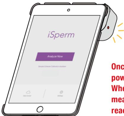
**Once the heater is connected to the power, LED indicator will turn on. When the LED starts flashing, this means that the temperature has reached  $37\pm 0.5$  °C.**
