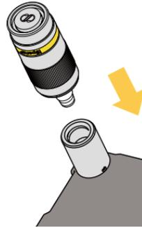
Screw the Sample Collector into the optical lens.
